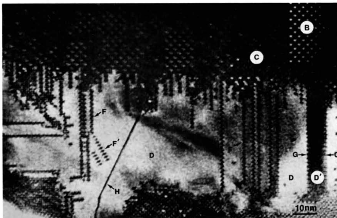
Fig. 1. Low-resolution lattice image from a fragment of nominal composition 17\text{Nb}_2\text{O}_5 \cdot 48\text{WO}_3 , showing the intergrowth between a tetragonal bronze host lattice (containing domains B of 2\text{Nb}_2\text{O}_5 \cdot 7\text{WO}_3 ), and second unresolved structure labelled D . The features labelled F , G and H are identified by the high-resolution data as rows of TTB elements, orientation boundaries, and a crystallographic shear defect respectively.
